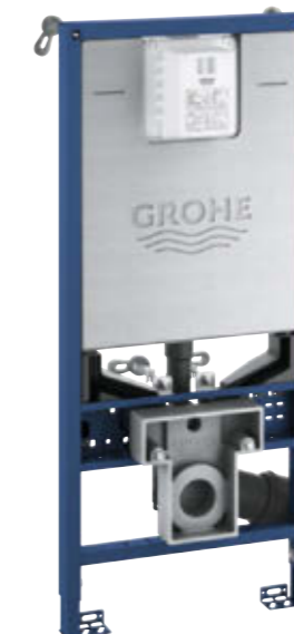
39 600 000 Rapid SLX WC 3-9 | 1.13 m SC Nordics adapter Rapid SLX Element for WC, 1.13 m installation height with flushing cistern GD2, with electric socket, including flow manager, easy access. Including pipe-in-pipe connection.
