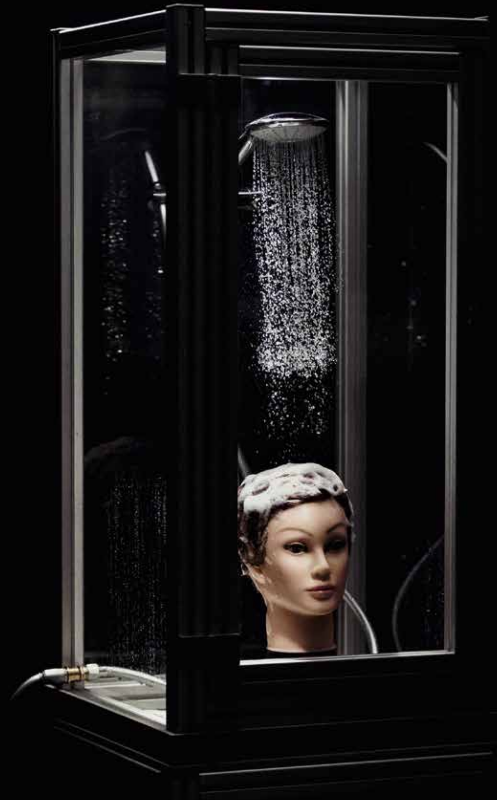
Bensing's shower lab examines shower head spray patterns, analyzing how they can be optimized to save water and increase efficiency.
