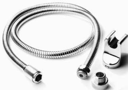
Cover :S.S 304 Germany cover Conctor : Pom Fitting : Brass Weight:330 gr Length : 1.20 Press : pom
