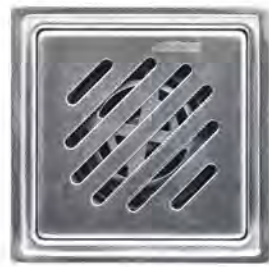
0305-21-79S1 Floor Drain SUS 304 Size 102*102 mm Height 57 mm Seal Type Self Seal ABS Flow Rate ≥15L/Min Outlet OD 42 mm Drain Core 0305-A1-7900
