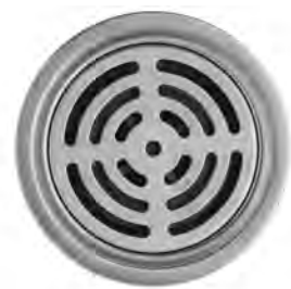
0305-04-79S1 Floor Drain SUS 304 Size 102*102 mm Height 57 mm Seal Type Self Seal Brass Flow Rate ≥15L/Min Outlet OD 42 mm Drain Core 0305-A1-7900
