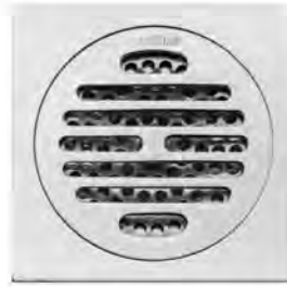
0303-62-79CP Floor Drain Brass Size 100*100 mm Height 43 mm Seal Type Self Seal Brass Flow Rate \geq 15L/Min Outlet OD 40 mm Drain Core 0303-A1-7900
