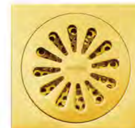
0303-61-79PK Floor Drain Brass Size 100*100 mm Height 43 mm Seal Type Self Seal Brass Flow Rate ≥15L/Min Outlet OD 40 mm Drain Core 0303-A1-7900
