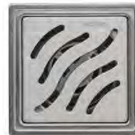
0305-19-79S1 Floor Drain SUS 304 Size 102*102 mm Height 57 mm Seal Type Self Seal ABS Flow Rate ≥15L/Min Outlet OD 42 mm Drain Core 0305-A1-7900
