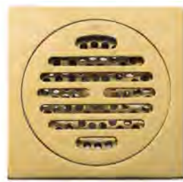
0303-62-79PK Floor Drain Brass Size 100*100 mm Height 43 mm Seal Type Self Seal Brass Flow Rate \geq 15L/Min Outlet OD 40 mm Drain Core 0303-A1-7900
