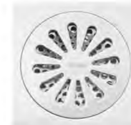
0303-61-79CP Floor Drain Brass Size 100*100 mm Height 43 mm Seal Type Self Seal Brass Flow Rate ≥15L/Min Outlet OD 40 mm Drain Core 0303-A1-7900
