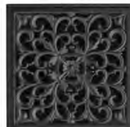
0303-71-79MA Floor Drain Brass Size 100*100 mm Height 61 mm Seal Type Self Seal Brass Flow Rate ≥15L/Min Outlet OD 40 mm Drain Core 0303-A1-7900
