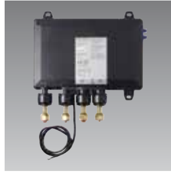
DTV Prompt thermostatic valve 340 x 318 x 68 mm 2 supply inlets G½ - 2 outlets G½ Portrait or landscape setting possible Flow depends on components - max 30 L/min via 1 outlet or 50 L/min via 2 outlets 528D-K-NA
